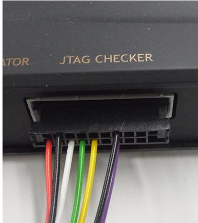
2. Connect the **JTAG cable** to the **target board connector**.
