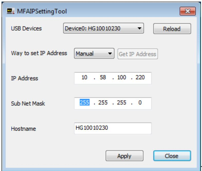
When you enter IP address, sub net mask and host name, jump to [“3.2.4 Write IP address settings to the Multifunction Analyzer”](#).
