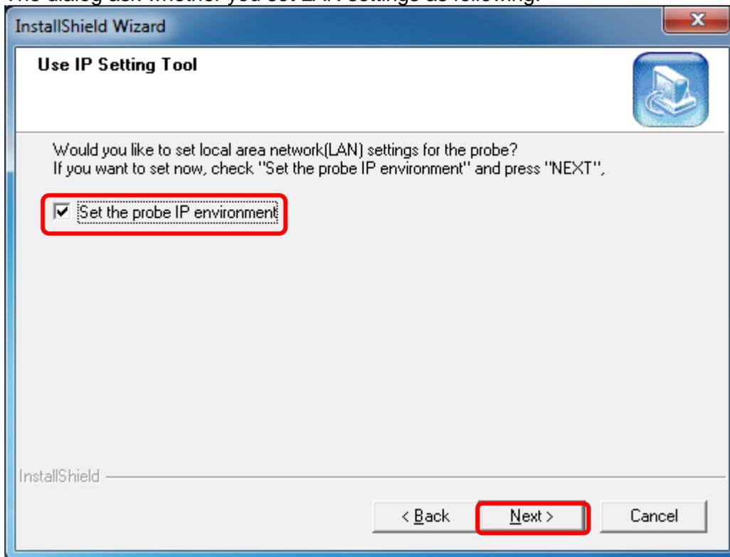
If you connect the Multifunction Analyzer to your PC with LAN without DHCP server, you have to set IP address and net mask manually.
