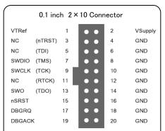
Recommended connector: 7620-6002 (3M) VTRef Vsupply Connect to Target power supply SCP7500: SCP 20 to 20
