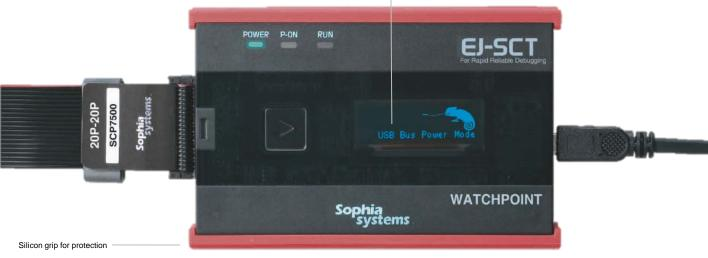
EJ-SCT is a development tool of a new era for general-purpose. Replacement of JTAG cables and the additional purchase of software licenses allow hardware support for debugging of all common variations of embedded CPUs. Including flash memory writing of program data.
