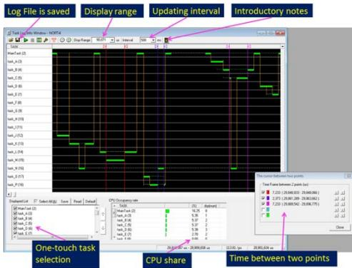
The OS task transitions display allows you to view time-series transition data for each task of OS and to review the occupancy rate of each task graphically. By profiling, it can be used as an indicator for the task flow optimization measures including improvement of task execution time and modification of the priority so that each task may be completed within the setting time. \*1
