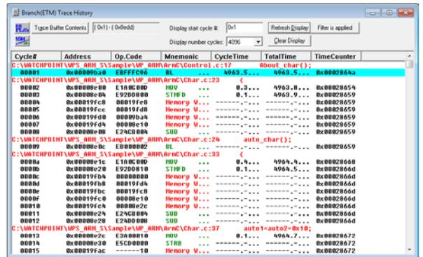
You can easily setup the trigger conditions and other conditions for trace in dialog box. The result of trace is displayed in special window. Supports ETM trace\*6, SWV trace\*7 and ETB trace \*6, \*7 Supported products: \*6: Cortex-M3, \*7: ARM series
