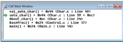
Double-clicking on a function name on the stack will open the Source window and display the calling source code.
