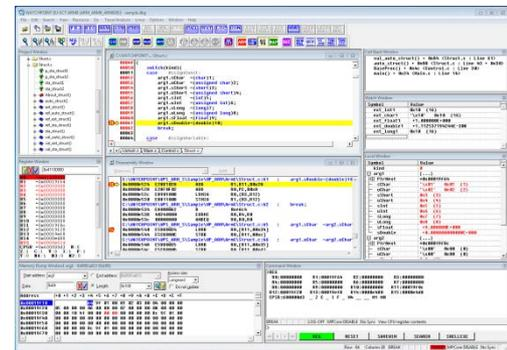
The child window inside WATCHPOINT (except for the source window) is available to be fixed by pasting to any of the four directions (sides) and to be placed on the outside of the main window.
