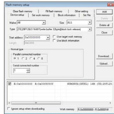
By only choosing a device of flash memory from pre-defined menu and set start address, the number of bit and the number of memory to be connected etc., you can download programs directly from debugger to flash memory on target system. It is not necessary to prepare another program such as software for flash programming or PROM writer. \*2
