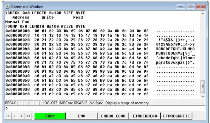
The command line interface allows you to control a debug session from the keyboard in addition to a debug control on Window GUI. Key in the first few letters of a command and Watchpoint will complete the command and its parameters. In addition, you can key in batch files for automatic execution and specify log files for saving the commands and results of a debug session.
