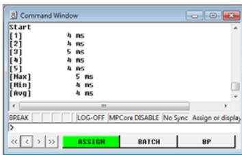
Easy Performance measurement records the CPU execution time for a specified range and can be used to measure the program execution time. The measurement cycle can be repeated a number of times, so Easy Performance measurement result displays each execution time along with an average of all execution cycle times. It can also record for CPUs that do not have trace capability. \*4
