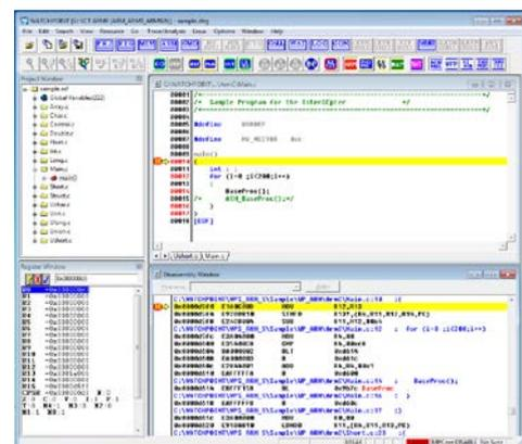
You can set hardware breakpoints in detailed hardware level such as breaks by access of memory or I/O. The number of software breakpoints is unlimited and it is possible to set to RAM or flash memory.
