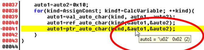
WATCHPOINT displays the current value when you position the mouse pointer over variable name in source program. It is useful to refer to the value without opening inspect dialog box.
