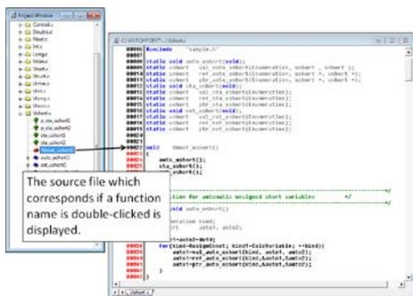
The project window displays the file name of currently downloaded module, the linked source-files and source file's functions, etc. in a tree format. Double-clicking on a source file name automatically opens a Source Window, and double-clicking on a function name automatically moves cursor to the location where the function is defined and displays the code, so you can quickly move onto specific areas of your code.
