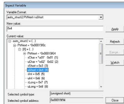
Double click on one variable in source window to view the contents of variable in a tree format. Embedded variables and member in complicated structures are also displayed. In addition, the variable value can be modified. The changes can be monitored in real time by registering the variable indicated in the inspect window into the watch window.
