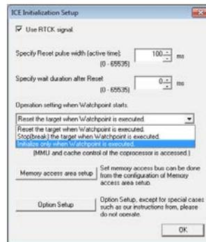
When using hot plug adapter together, you can start WATCHPOINT (WP) without reset of CPU, and can start debugging smoothly after a problem occurs. \*5
