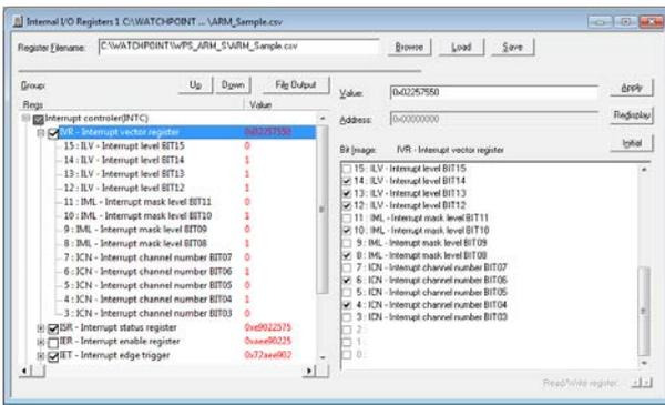
You can view and modify the CPU internal resources (MMU registers, internal I/O registers etc.). Register name, register value and also bit value of each register are displayed in a tree format. Programs can be executed while opening the internal register window. It is helpful to debug while monitoring the status of interrupt and timer.
